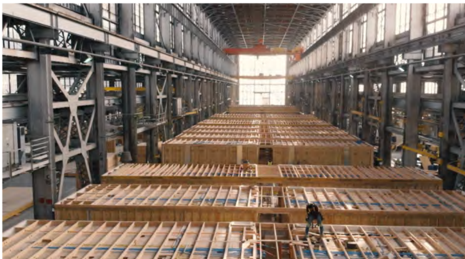
Overview of modules moving through the assembly line. Image courtesy of Autodesk.
